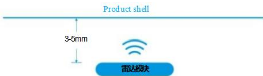
Figure 9 Distance between antenna surface and product shell
